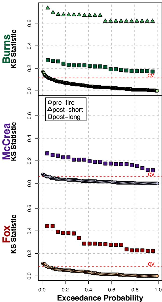
**FIGURE 4** Kolmogorov–Smirnov (KS) test statistic versus exceedance probability between pre-fire (1961–1970) median flow duration curves (FDC) and post-short (1971–1977) and post-long (2005–2011) jackknifed FDCs across Burns, McCrea, and Fox Creeks. The critical value (cv), indicated by the red-dashed line, was based on the pre-fire 0.05 Weibull plotting position. McCrea and Fox Creeks post-short were not included due to insufficient years for jackknife resampling
